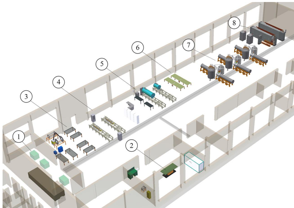
Figure 1: Schematic 3d-view of the facility halls and main equipment placement: 1 – Nuclotron-type SC cable production hall; 2 – magnets windings production hall; 3 –assembling the yoke of the magnet and winding, welding and brazing cooling channels of magnets; 4 –room temperature magnetic measurements; 5 –check vacuum tightness of cooling channels, beam pipes and cryostats; 6 –assembling magnets in cryostats; 7 –cryogenic tests of magnets at 6 benches; 8 –power converters hall.
