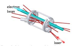
Figure 3: Schematic drawing of the enhancement cavity.
