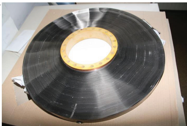
Figure 1: One final ring core made of magnetic nano-alloy ribbon (Nanoperm of Magnetec; diameters: 500mm/200mm, height: 30mm).
