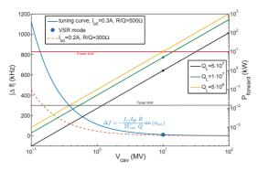
Figure 1: Optimum tuning curve for reactive beam-loading for the VSR (blue curve) and a lower R/Q-reduced intensity scenario (brown curve) as well as the required power with optimum detuning for different  $Q_L$ . Limits of the tuner and power source are given by the horizontal lines.
