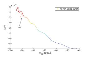
Figure 6: Example of DC Robinson instability caused by a too low feedback gain of  $K_{\rm P}$ =35.
