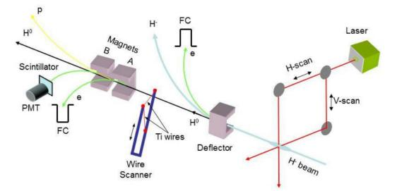
Figure 1: Schematic of laser wire based  $H^-$  beam emittance measurement system. FC: Faraday cup, PMT: photomultiplier tube, Magnets A and B deflects electrons for FC and scintillator detection schemes, respectively.
