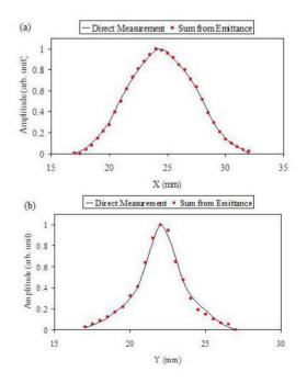
Figure 4: Comparison of directly measured profiles (blue lines) and profiles integrated from the emittance distributions (red dots). (a) Horizontal and (b) vertical profiles.
