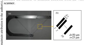
must 1 Figure 2: (a) Photo and (b) schematic diagram of the 10string titanium wire scanner.
