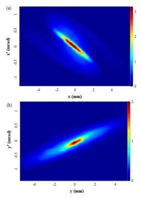
Figure 3: Emittance measured using the 10-string wire scanner and the Faraday cup electron collector scheme.
