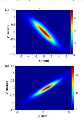
Figure 6: Emittance measured using the scintillator-PMT detection scheme.
