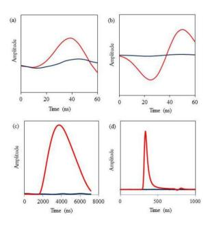
Figure 5: Output waveforms from the titanium wire scanner. Red and blue lines correspond to signals at the center and edge of the emittance plot. (a) single-string wire scanner output, (b)-(d) 10-string wire scanner outputs at different detection schemes.
