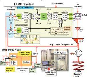
Figure 4: Setup of high power test of KLY-PLL and beam loading test using ARES cavity simulator.
