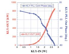
Figure 5: Klystron input-output characteristics measured under closed loop of the I/Q-FB control with the KLY-PLL control.
