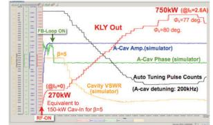
Content from this work may be used under the terms of Figure 6: The chart of beam loading simulation test by using ARES cavity simulator under the closed loop for the cavity-voltage regulation control with KLY-PLL.
