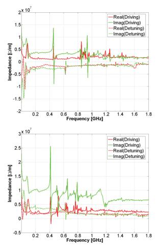
Figure 1: Horizontal (top) and vertical (bottom) SPS impedance model.
