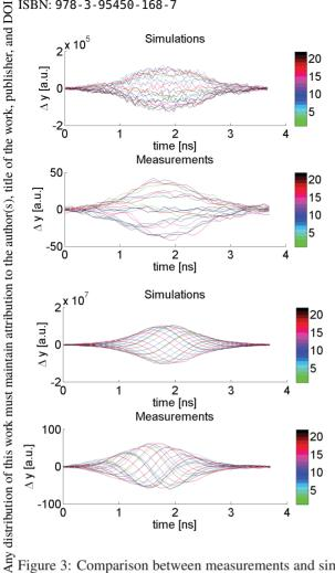
Figure 3: Comparison between measurements and simulac tions of the intra-bunch motion over 21 consecutive turns of for  $\xi = -0.067$  (top) and  $\xi = -0.967$  (bottom).
