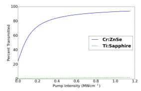
Figure 3: Left:The gain for either a Cr:ZnSe or Ti:Sapph crystal with 2 mm signal delay as a function of intensity. Right: Transmission of pump laser for a CrZnSe and Ti:Sapph crystal.
