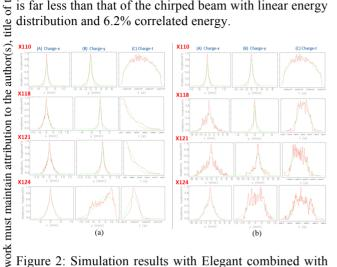
Solution Figure 2: Simulation results with Elegant combined with Shower (Q = 3.2 nC and 50 MeV). Bunch profiles (a) without and (b) with a slit-mask at X115.
