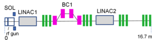
Figure 3: Overview of the ATF upgrade photo-injector. SOL is the solenoidal lens, LINAC 1, LINAC2 are the 2.856 GHz SLAC sections. BC1 is the bunch compressor chicane.
