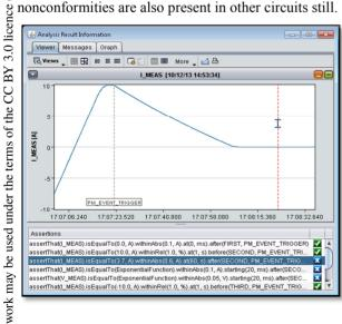
Figure 2: Current discharge curve of a 60A orbit corrector circuit with a faulty crowbar resistance not from 1 revealed during 3 previous (manual) analysis campaigns.
