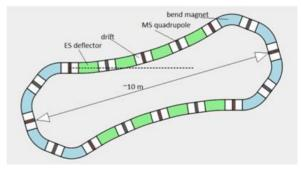
Figure 2: Ring lattice based on QFS concept.
