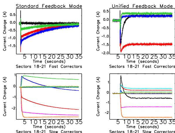
Figure 2: Vertical fast and slow corrector step response comparison between unified and standard feedback.
