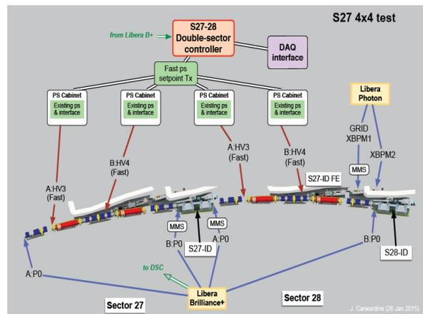
Figure 1: MBA diagnostics integrated R&D in APS storage ring sector 27. The P0 labels are ID BPMs and the HV labels are fast correctors.
