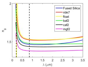
Figure 3: Group index for six different glasses. Dotted lines bracket the streak camera spectrum: [200-850nm].
