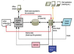
Figure 1: Online Model Platform schematic diagram.
