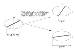
Figure 1: Adjusting the horizontal beam size [2].
