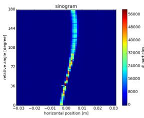
Figure 6: Sinogram of the measured projections
