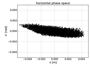
Figure 3: Simulated horizontal phase space.
