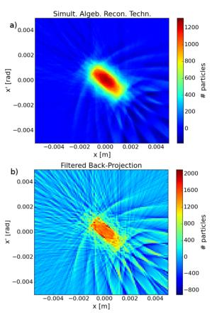
Figure 7: Reconstruction using a) FBP and b) SART.
