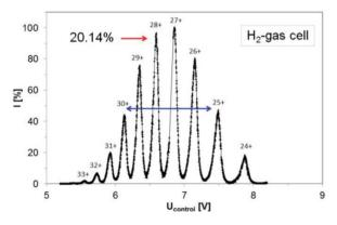
Figure 2: N<sub>2</sub>-gas jet (top) and H<sub>2</sub>-pulsed gas cell (bottom) charge spectra for max. available target density [13].
