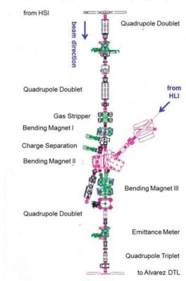
Figure 1: Layout of the 1.4 MeV/u stripper section; 14.0 m total length.
