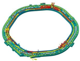
Figure 1: Design of T110, including the accelerator tunnel (outer tunnel) and the parallel supply tunnel (inner tunnel) with cable trays (yellow), cooling water supply lines (blue) and venting (red).
