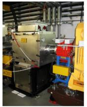
Figure 5: SIS18 MA loaded bunch compression cavity.
