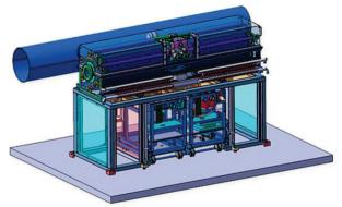
Figure 4: GSI design of the ferrite loaded acceleration cavity.
