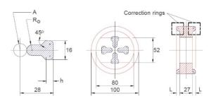
Figure 2: The electrodes with carrier and correction rings [4]
