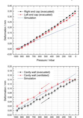
Figure 4: Measured deformation of the end caps (top) and of the cavity wall (bottom) at 1 bar pressure difference.
