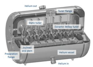
Figure 1: Layout of the sc 217 MHz CH cavity.
