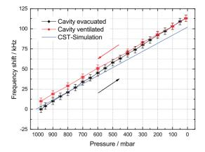
Figure 5: Measured frequency shift due to evacuation.
