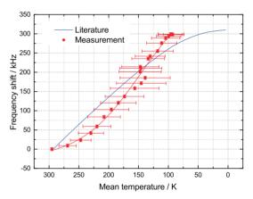
Figure 7: Frequency shift due to cavity shrinkage.
