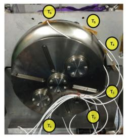
Figure 6: Position of the temperature probes.
