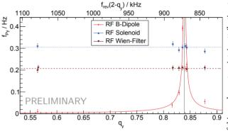
Figure 5: Results of the resonance scans at the nominal tune of COSY at  $Q_y = 3.56$  and for a set of vertical betatron tunes with sideband frequencies around the spin resonance depicted by the vertical line at  $871428.00 \, \text{Hz}$ .
