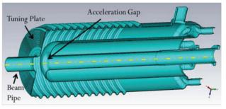
Figure 2: Crossection view of the 56 MHz SRF cavity.
