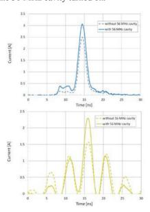
Figure 7: Beam profile comparison for 56 MHz cavity turned on and off. Top: Blue ring with He3 particles. Bottom: Yellow ring with Au particles.
