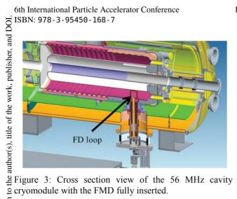
2 cryomodule with the FMD fully inserted.
