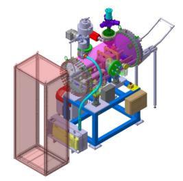
Figure 3: Test tank for the HESR injection kickers as to be delivered to the contractor. For detailed description see text.
