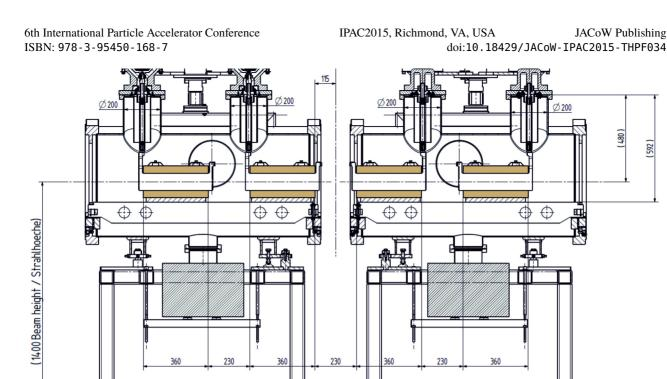
Figure 2: Mechanical layout of the injection kickers including vacuum tanks. During bake-out the termination resistors (top, not completely shown) can be disconnected and lifted without breaking the vacuum.
