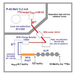
Figure 1: Functional scheme of the SPES facility. There are two main areas: the 1+ line and the n+ line, where 1+ and n+ indicates the beam charge state.
