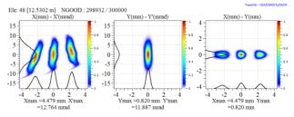
Figure 3: Phase space at the HRMS image point. The three beams are separated of 1/20000 with  $\pm$  1eV energy spread.
