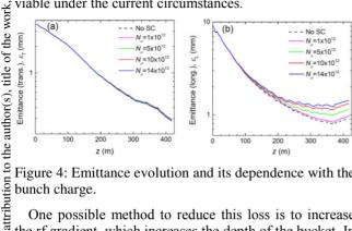
Figure 4: Emittance evolution and its dependence with the bunch charge.
