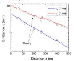
Figure 3: Cooling performance vs. distance. Solid lines are simulation results and circles are results from theory.
