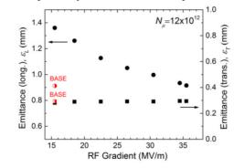
Figure 5: Final emittance achieved vs. gradient for a given space-charge intensity.
