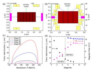
Figure 1: Lattice characteristics of the proposed rectilinear 6D cooling channel: (a) Early stage, (b) last cooling stage, (c) beta function for different stages, and (d) beta and maximum axial field per stage as well as allowable field limit for Nb<sub>3</sub>Sn.
