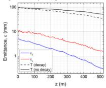
Figure 6: Emittance and transmission evolution in a hybrid cooling channel with gas filled cavities.
