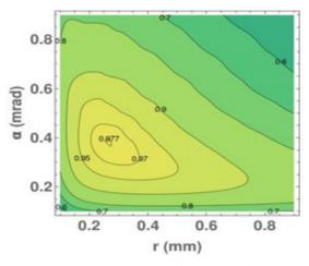
Figure 5: Laser excitation efficiency as function of r and  $\alpha$  of the laser beam parameters. The maximum excitation locates at 0.26 mm and 0.39 mrad for r and  $\alpha$ , respectively.
