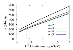
Figure 3: Doppler shift of the transition wavelength of  $H^0$  as a function of its kinetic energy is calculated by using Eqn. 1. n is the principal quantum number of hydrogen atom. Laser wavelength for 400 MeV is required to be 230 nm.
