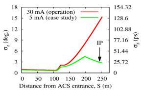
Figure 4: Simulation results for the 400 MeV longitudinal  $H^-$  beam size in the J-PARC Linac.
