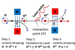
Figure 1: Schematic view of laser-assisted H<sup>-</sup> stripping.
