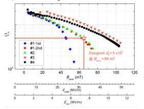
Figure 3: VT results of the spoke021 cavities.
