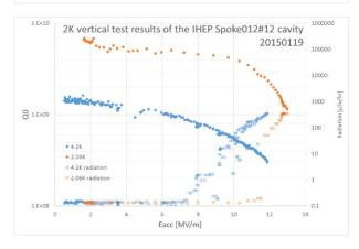
Figure 2: VT results of the spoke012 cavities.
