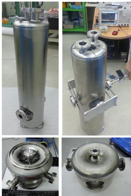
Figure 4: Photographs of prototype superconducting cavities [QWR(top left), HWR(top right), SSR1(bottom right), SSR2(bottom left)].
