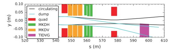
Figure 4: Schematic side view of the SPS dump system in LSS5 using three MKDVs. In cyan the  $\pm 3.5\sigma_y$  14 GeV FT beam envelope is plotted corresponding to the vertical acceptance of one of the main SPS dipole families.
