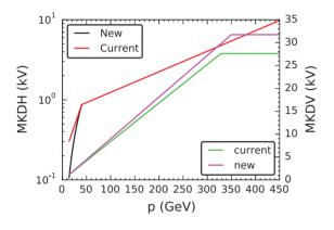
Figure 5: New proposed energy tracking functions for the MKDV (magenta) and MKDH (black, in logarithmic scale). The comparison is made for the equivalent of the current system but with three MKDVs, and the LSS5 option.
