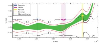
Figure 2: Proposed extraction channel in LSS5 using the same elements as in LSS4. In green the envelope of the last three turns trajectory of the particle with the maximum allowed amplitude at the extraction electrostatic septum ZS2 is shown. In red the beam envelope calculated as  $A(s) = (D\delta_p + 1.2 \times \max\{6\sqrt{\epsilon \beta}, x_{3turns}\})1.1 + 6mm$ .
