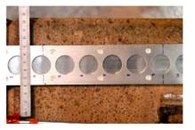
Figure 1: Gold foil array used in the measurements.
