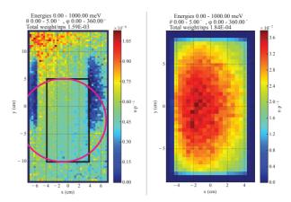
Figure 3: The thermal neutron current distribution in a  $5^{\circ}$ cone normal to the EIGER-facing surface water scatterer (left) and the downstream surface of the sapphire crystal (right). The solid magenta curve shows the approximate view of the EIGER nozzle and the solid black rectangle shows the approximate view of the of sapphire crystal.
