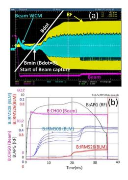
Figure 5: A measurement data on early injection scheme: a) Scope data for the first 1 ms after beam injection (pink trace is -1×Beam) b) 13BT beam, total RF voltage and loss monitor data from injection to extraction without notch in the beam. The beam efficiency was nearly 94% in this case.
