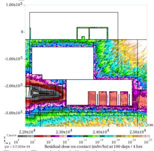
Figure 4: The calculated distributions of prompt (top) and residual (bottom) dose around the facility at normal operation at 120 GeV.
