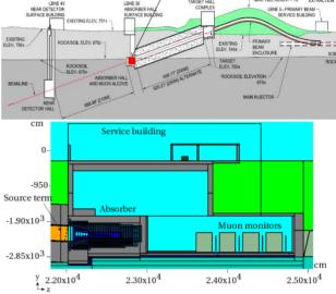
Figure 1: Elevation view of the entire facility (top) and a fragment of the MARS model that shows the hadron absorber and muon monitors in the hall with a service building above (bottom).
