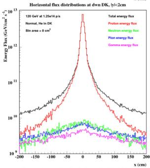
Horizontal energy flux distributions at dwn DK, |y|<2cm Figure 2: Incoming particle (top) and energy (bottom) flux at absorber for normal operation at 120 GeV with helium in the decay pipe.
