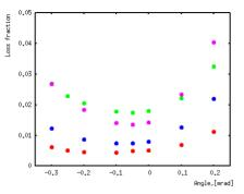
attribution to the author(s), title of the work, Figure 6: Fraction of the local and total beam loss versus the incident angle of the beam with respect to the septum plane. 50µ W foil strips plane: purple points – total losses and blue points- local losses; 100 µ diameter W wire plane: green points- total losses and red points- local losses. must 1
