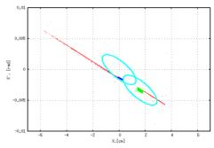
Figure 5: Phase space of the beam at the C-magnet exit after scattering in the ESS foils.
