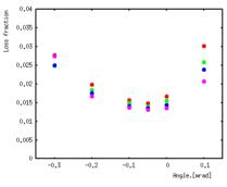
the terms of the CC BY 3.0 licence (© Figure 7: Total loss fraction versus beam incident angle misalignment for various ESS1/ESS2 lengths: red points: L1/L2= 1.5m/1.5m; green - L1/L2= 1.0m/2.0m; blue- $\frac{1}{2}$  L1/L2 = 0.7m/2.3m; purple- L1/L2=0.5m/2.5m.
