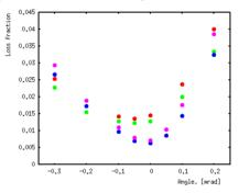
Figure 8: Fraction of total beam losses in the foil strip septum with a 30cm long carbon foil strip diffuser in front of the septum plane (blue - Mo foils, purple - W foils) and without pre-scattering (green – Mo foils, red - W foils).
