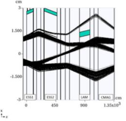
Figure 4: Tracking the multiband sample in the extraction channel –horizontal plane view. The upper band shows part of the extracted beam closest to the septa planes. The other three bands show the boundary of the circulating beam envelope.
