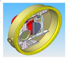
Figure 6: Design of the movable frame for the SA (front) and the lead radiation shutter (back). The half discs of lead shutter (grey) can be seen together with the rails inside the MICE vacuum chamber (yellow).
