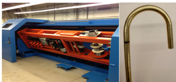
Figure 4: a) Continuous tube forming of the sheath tube; b) specimen of CIC cable bent to the radius required for the windings of the 4.5 T dipole.
