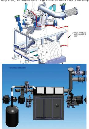
Figure 6: Top: The components of the liquid lithium stripper are shown. The pump is in the forefront. Bottom: we show the steel secondary containment vessel (2 m long) that will remain full of Ar. A vent to a scrubber is shown on the upper right and the Ar supply tank on the lower left.
