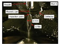
under the terms of the CC BY 3.0 licence ( Figure 2: Liquid lithium film formed by impact of a high velocity jet on a deflector at the ANL lithium test stand p velo [6].
