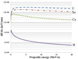
Figure 1: Comparison of the energy loss per unit length in carbon foils for some heavy ions and protons. A single U ion deposits three orders of magnitude higher power than a proton of the same velocity. Stripping energies at FRIB are between 16 and 20 MeV/u.
