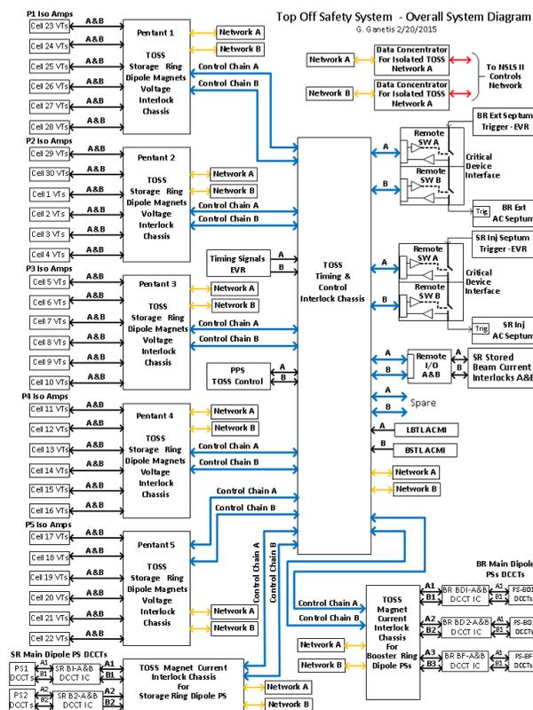
Figure 3: Schematic diagram of the TOSS. Blue lines denote safety related communication, yellow is non-safety diagnostic information, and black is raw signal.
