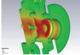
Figure 7: Choke structure of cathode rod.
