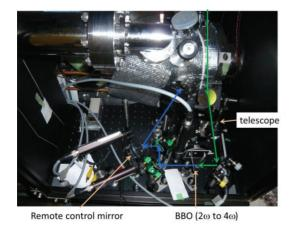
Figure 3: Optics for laser injection.
