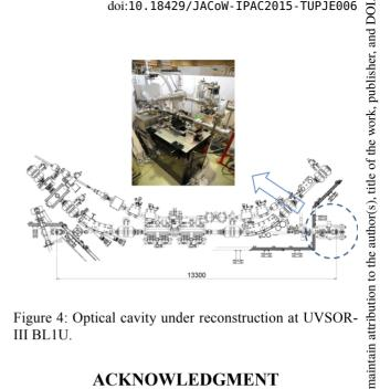
Figure 4: Optical cavity under reconstruction at UVSOR-III BL1U.
