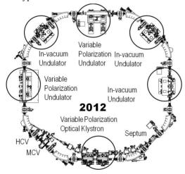
Figure 2: Configuration of UVSOR-III [24].
