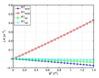
Figure 2: K1 values for compensating tune shift and matching beta function for WIG.
