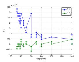
Figure 5: Residual tune shift after compensation.
