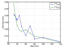
Figure 6: Residual orbit distortion caused by WIG.
