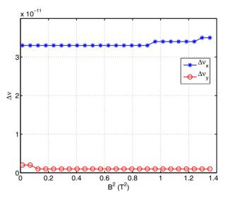
Figure 3: Residual tune shift after compensation.
