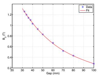
Figure 4: Measured  $B_0$  as a function of the magnet pole gap of WIG.
