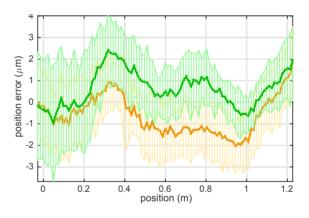
Figure 2: Longitudinal position error (real with respect to encoder reading), forward (orange) and backwards (green). Thick lines link mean values, light lines the associated dispersion.
