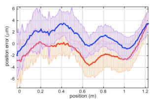
Figure 3: Straightness (horizontal error) along z axis forward (red) and backwards (blue). Thick and light lines have same meaning as above.
