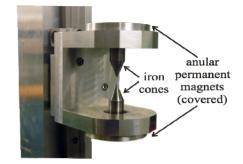
Figure 6: Cone system used to fiducialize Hall probe head.
