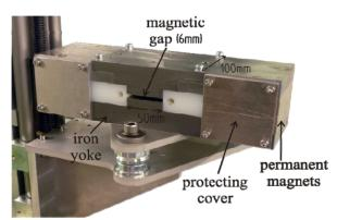
Figure 5: Reference dipole magnet made at CELLS.
