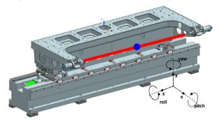
Figure 1: General view of the new Hall probe bench and reference system. Stretched belt is painted red, and Hall probe position is marked with a blue dot.
