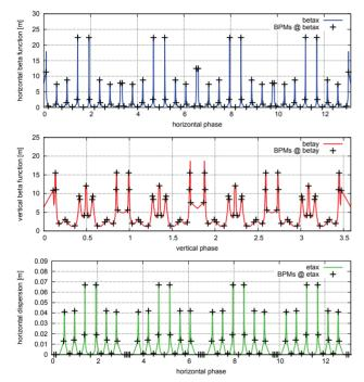
Figure 2: Photon and RF BPM layout with 20 photon and 64 RF BPMs for one 3rd of SLS-2. BPMs are visualized as "+" with the values of the corresponding beta functions and horizontal dispersion, where the total phase advance of SLS-2 (Version AD05F) is 39.417 and 10.755.
