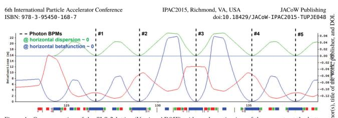
Figure 1: One arc section of the SLS-2 lattice (Version AD05F) with a schematic view of the magnets at the bottom (dipole magnets in blue) and the optical functions. The horizontal beta function (blue) and the horizontal dispersion (green) vanishes in the center of the bending magnets in order to provide small horizontal emittance. Five additional photon BPMs (#1-#5) have been added in the center of the main bends for improved orbit sampling.
