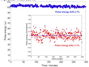
Figure 5: Laser pulse energy variation delivered by the VELA photoinjector laser and transport system to the photocathode, measured over a typical operating period of six hours (main figure, blue; 10 minute average, red) and over 350 shots (at 10 Hz) Both the long and short Sover 350 shots (at 10 Hz). Both the long and short  $\stackrel{\scriptstyle{\leftarrow}}{=}$  variation is within 1 % of the pulse energy. 2015).
