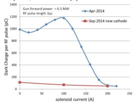
Figure 3: DC measured on WCM-01 with the original (April 2014) and new (Sep 2014) photocathode.
