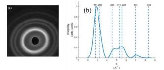
Figure 6: (a) 1000 shot accumulated diffraction pattern of polycrystalline platinum, and (b) Azimuthal integration of polycrystalline platinum diffraction with expected diffraction peaks overlaid as dashed lines.
