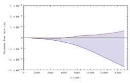
Figure 3: X projection of the trajectories of 150 GeV electrons travelling through simulated 1.7825 m long undulator modules with a nominal magnetic field strength of 0.88 T. The band shows the average trajectory +/- 1 standard deviation as calculated from 20 simulated field maps.
