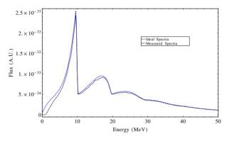
Figure 4: Calculated energy spectrum from tracking a single electron through a 1.7825 m long undulator with a circular aperture with a radius of 0.0045 m at a distance of 500 m from the end of the undulator. The blue dashed line shows the result from an ideal map, and the black dashed line shows the result from the measured map.
