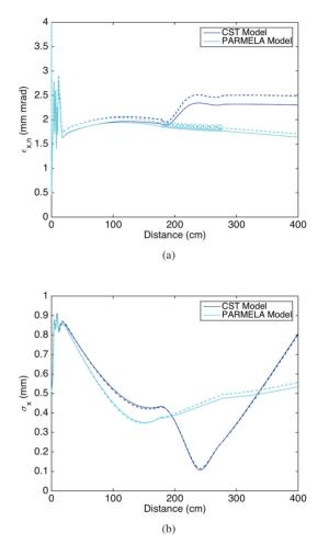
Figure 3: a) Transverse normalised emittance and b) the beam size as a function of the distance from the cathode. (Solid and dashed lines are x and y axes, respectively.)
