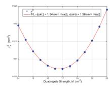
þe Figure 6: A simulated quadrupole scan result in the postmay booster region.
