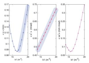
Figure 7: Beam size, divergence and the correlation terms for the range of working points of the injector.
