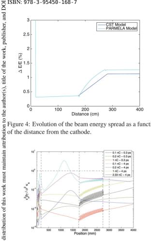
Figure 4: Evolution of the beam energy spread as a function of the distance from the cathode.
