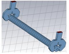
Figure 2: A snapshot from CST design of the S-band travelling wave structure as the energy booster linac for the electron injector.
