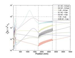
Figure 5: The ratio of space charge and emittance term of the beam envelope as a function of the distance from the 2015). cathode.
