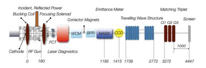
Figure 1: The layout of the photo injector and the booster linac section to provide a witness beam for the AWAKE plasma wakefield acceleration experiment.
