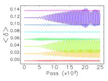
Figure 4: Momentum centroid oscillations for 8 realizations of 120 randomized HOMs. Data is staggered for clarity.
