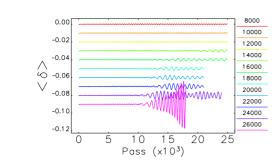
Figure 2: Momentum centroid oscillations for different O author(s). values of the 540-MHz HOM. Data is staggered 0.01 units vertically for clarity. Time coordinate centroid oscillations would show essentially the same thing. the
