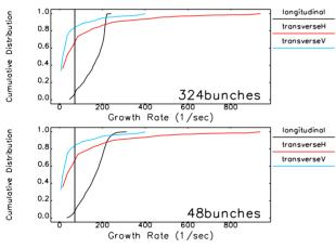
Figure 1: Cumulative distribution function of the maximum growth rate for symmetric bunch patterns. The black line shows longitudinal damping rate.
