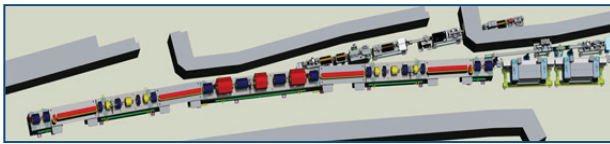
Figure 1: Layout of one APS-U sector. Dipole magnets are shown in red, quadrupole magnets in blue and sextupole magnets in yellow.
