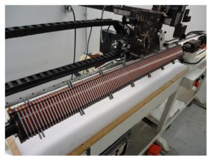
Figure 1: SCU1 magnet core on winding machine.
