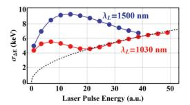
Figure 2: Energy spread at the entrance of L1 (two choices of laser wavelengths) showing evidence of the 'trickle' heating effect;  $\sigma_E = 0.1$  keV. The dashed line is the nominal heating in the absence of collective effects.
