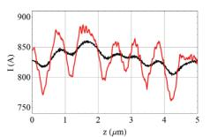
Figure 7: The beam current profile as seen at the entrance of DL1 (black curve) shows ~ 1% longitudinal bunching amplitude at about  $\lambda \simeq 1 \ \mu m$  wavelength. By the exit of the dogleg (red curve) bunching has grown to about 4%, implying a net ~ 3% contribution from TSC in the dogleg. The quoted numbers are about the middle of the observed value ranges.
