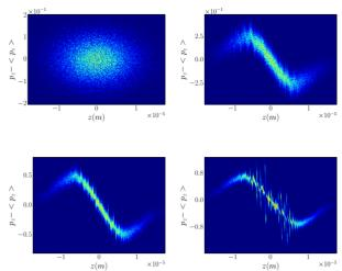
Figure 2: Snapshots of longitudinal-phase space evolution along the cascaded LSCA: initial (Gaussian) bunch before (top left) and after passing through one (top right), two (bottom left) and three (bottom right) LSCA module. The Lorentz factor is  $\gamma = 670$ .
