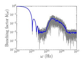
Figure 3: Comparison of averaged bunching factor (blue trace) with bunching factors computed using 100 independent realizations of the initial bunch distributions (gray traces).
