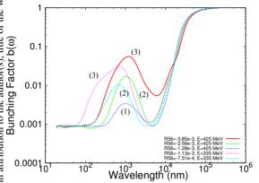
Figure 4: Average bunching factor for various cases of  $R_{56}$  and beam energies (see legend). Spline interpolation has been applied. The number in brackets indicates after which LSCA module the bunching factor is evaluated.
